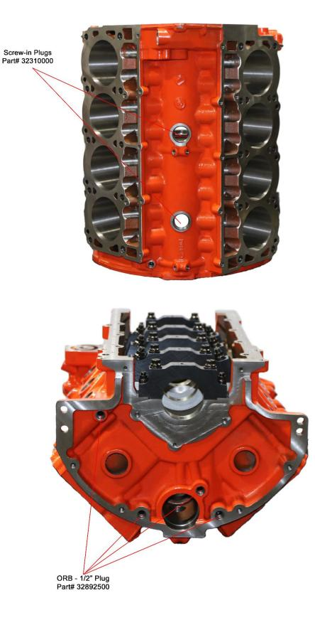
**SPECIAL NOTES FOR NON-VVT BLOCKS ONLY:** Use a ¼" NPT - .333" OAL plug (Part# 32890250S) in the front oil galley threaded port. Using a longer plug may cause it to extend into the main oil galley feed port, leading to oiling issues and potential engine failure.
