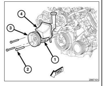
8. Install the pressure line (2) on the pump (3) and tighten the power steering nut to 38 N·m (28 ft. lbs.). Fitting size for pressure line is M16x1.5.
