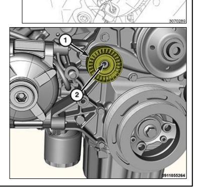
6. Align the locator tang and install the belt tensioner. Tighten the tensioner bolt (3) to the proper torque specification 55 N·m (41 Ft·Lbs).
