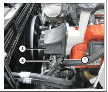
NOTE: When installing accessory drive belt onto pulleys, make sure that belt is properly routed and all V-grooves make proper contact with pulleys.
