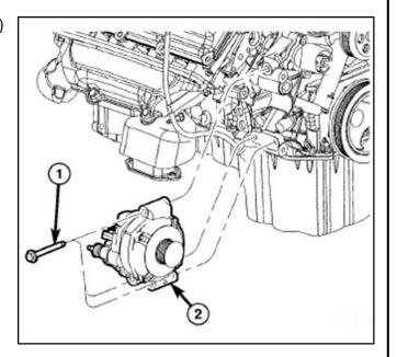
2. Position the generator B+ terminal eyelet to the generator output stud, install the retaining nut (3) and tighten to the proper torque specification 14 N·m (10 Ft·Lbs).
