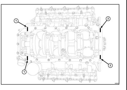
**NOTE:** When the oil pan is removed, a new integral windage tray and gasket assembly must be installed. The old gasket cannot be reused.
