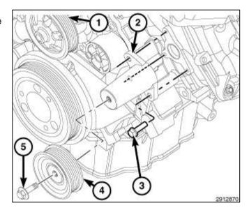
Position the power steering pump (1) and using the holes in the pulley for access, install 3 pump mounting bolts (5) and tighten to 23 N·m (17 ft. lbs.).
