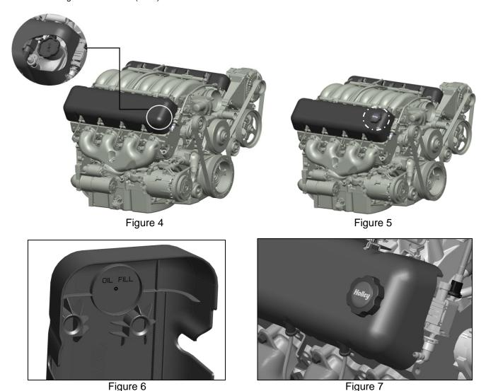
Install the (x10) snap grommets in bottom side of cover's sockets (**Figure 6**). After installing each grommet, rotate it in the socket to confirm it is fully seated.
