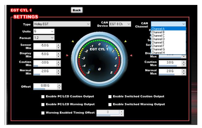
3) Select the Proper CAN Bus Channel. "CAN BUS 1" is the connector on the main harness. "CAN BUS 2" is on the J3 connector available only on dominators.
