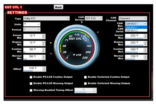
4) Select the "CAN Serial" that matches your controller. This is a unique number and will be differenct on each controller. It can be found on the bottom sticker of the controller.
