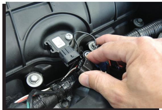
**Figure 5 Disconnect the MAP Sensor.**
