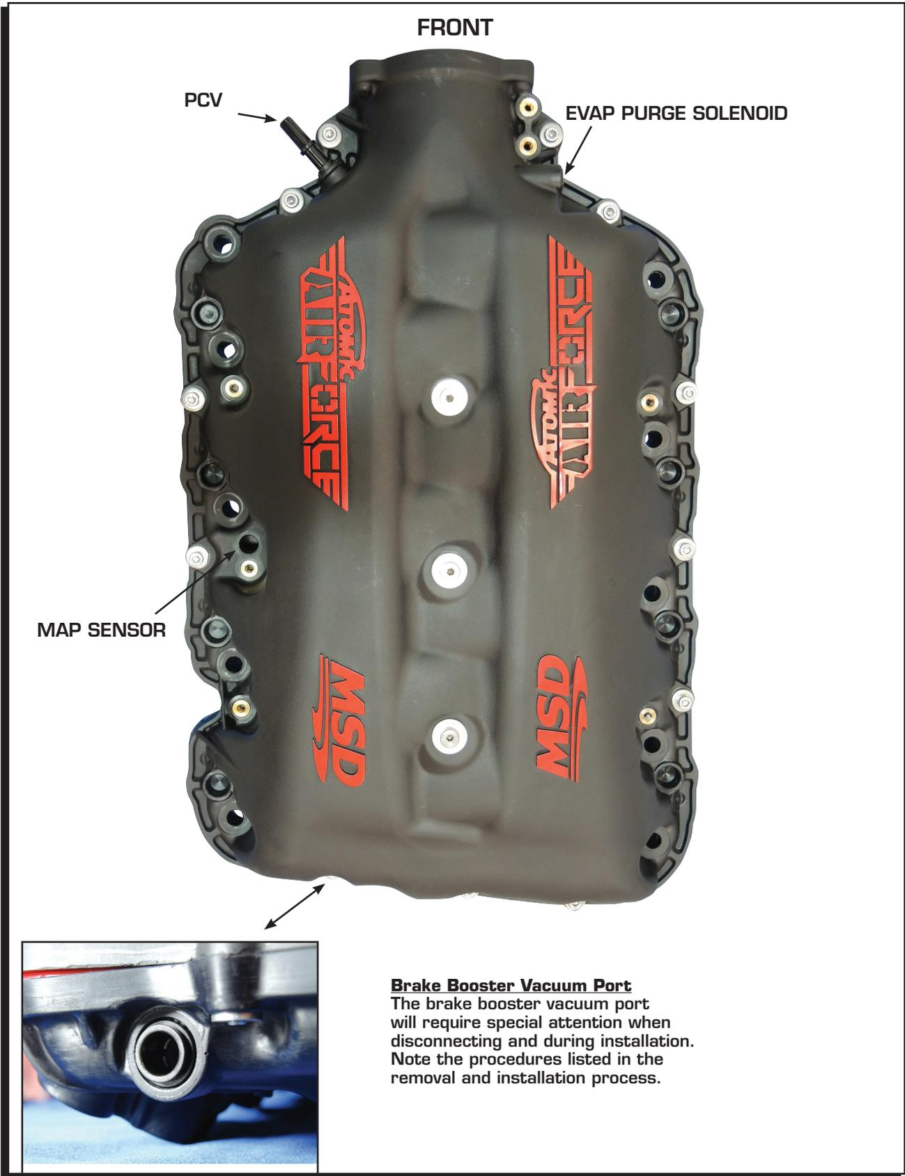
Figure 1 Vacuum Ports of the AirForce LT1 Manifold.
