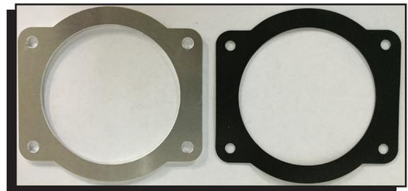
**Figure 14 TB Seal Plate and Gasket**
