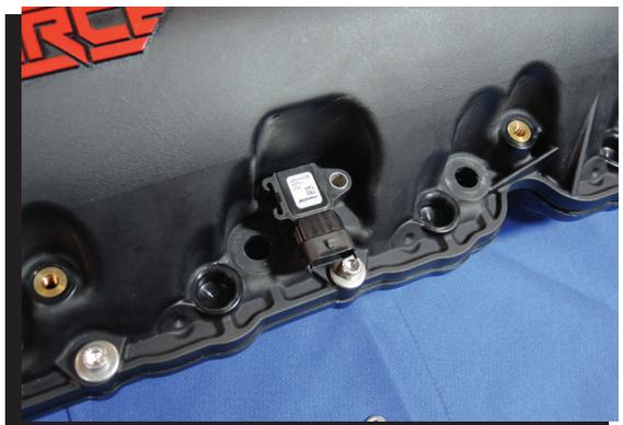
Figure 8 Install the MAP Sensor.
