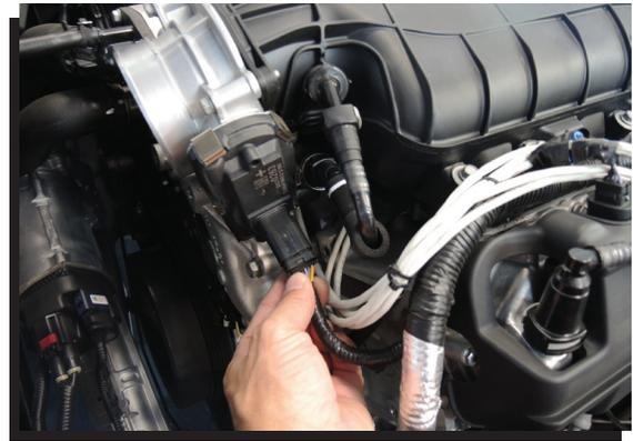
**Figure 2 Disconnect the ETC.**
