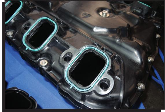
**Figure 11 Install the Port Seals.**
