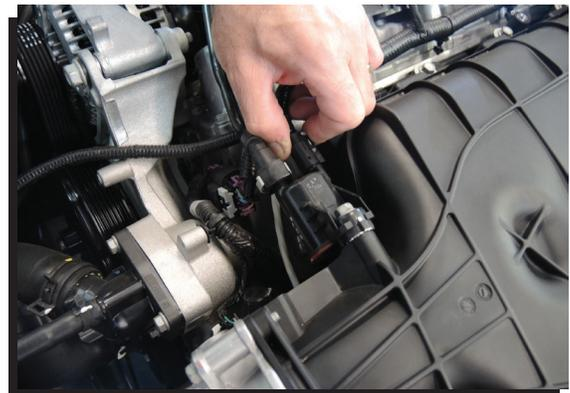
**Figure 3 Disconnect the EVAP Solenoid and Tube.**
