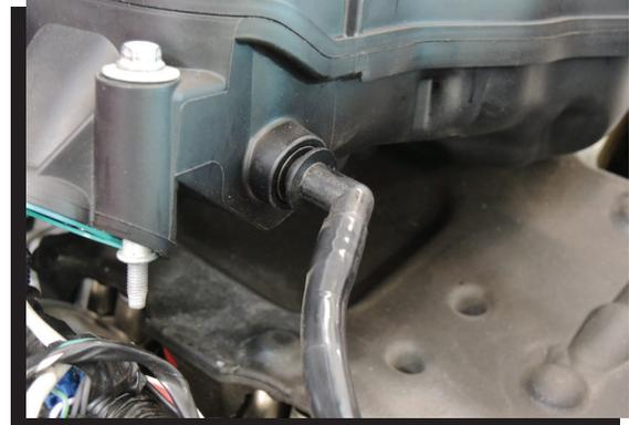
Figure 6 Brake Booster Vacuum Connection.
