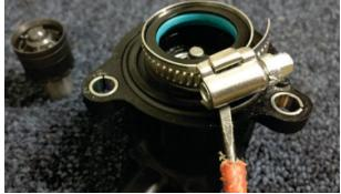
Pull the piston and spring out of the body, then remove the o-ring (keep this safe, it will be re-used in the DV+ installation). The remaining black plastic protrusion and blue piston ring MUST BE REMOVED before the DV+ is installed.
