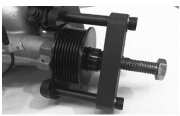
2. Using a pulley removal tool, such as the Lingenfelter L950066509 pulley removal tool shown to the left, remove the factory pulley from the supercharger front cover.
