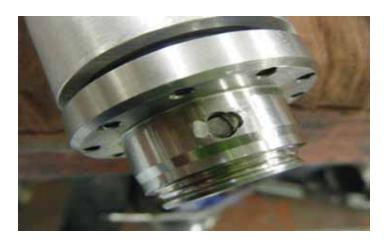
11. Secure the front cover and supercharger pulley. Using a hammer and punch, hit the two surfaces around the pin shown to the left. This will keep the dowel pin securely in place.
