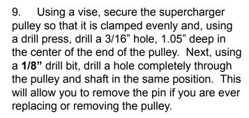
**NOTE:** LPE recommends using a hardened solid carbide drill bit to drill the 3/16" hole as the shaft material is very hard.
