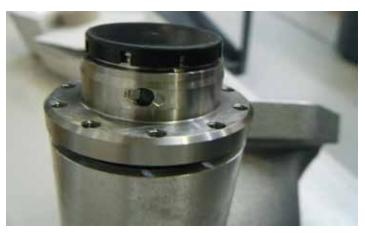
12. Reinstall the black cap onto the front of the hub.
