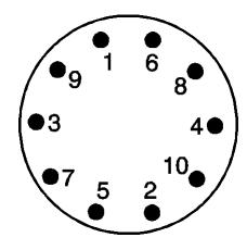
14. Apply a small amount of Loctite Blue to the supplied M4x0.7x12 socket head cap screws and, using a 3 mm Allen wrench or socket, secure the pulley to the hub with these screws. Use the pattern to the left to tighten the screws. Torque to 2.3 Nm (20.7 lb-in).
