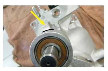
4. Start by marking both of the tabs with a black marker. Make sure that the you do not go below your mark in the machining process. LPE suggests using an adjustable boring head or a die grinder to remove material. Remove the tabs 1.55" down as illustrated in the next step.
