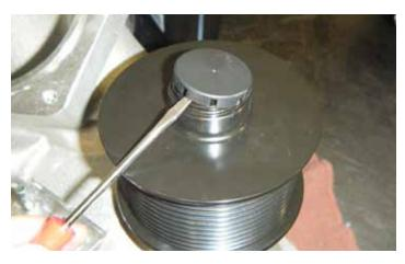
1. Remove the cap on the pulley by using a small flat head screwdriver and prying up.
