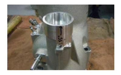
5. Using a runout gage, locate your end mill to be concentric with the inside of the jackshaft housing (you may also use the jackshaft itself to center the endmill). You can complete the machining with the jackshaft installed if your boring gage allows it, otherwise you will need to remove the jackshaft. If you remove the jackshaft, you must replace the bearings. See the next step for the dimensions of the machined part.
