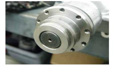
Steps 8-10 are optional. Since the supercharger pulley is spinning at higher RPM and driving more load than the stock pulley, pinning the pulley is recommended but not required. LPE pins all of their LSA & LS9 supercharger pulleys.
