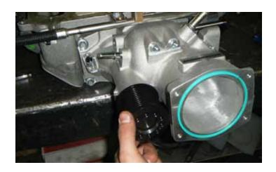
13. Install the supercharger pulley onto the 10 bolt hub.
