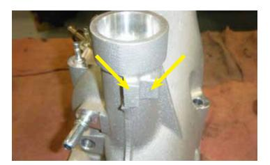
3. Steps 4-6 will detail the machining operation that must take place in order to provide enough clearence for the new pulley.
