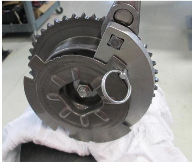
**Step 6:** Using the included TORX Plus bit, locate the pivot bolt and loosen it 1/2 turn. It is the first bolt located clockwise from the pin-bolt. Remember, DO NOT remove this bolt, just loosen it 1/2 turn. Remove the other four bolts and temporarily remove the safety bolt. Rotate the cover away to expose the phaser control chambers.
