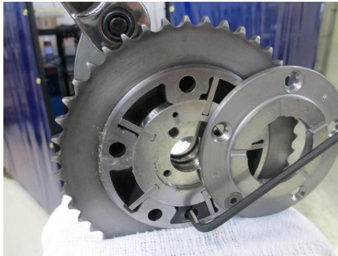
**Step 9:** Rotate the cover plate back over the control chambers and reinstall the safety bolt. Reinstall the cam phaser bolts, making sure to install the pin-bolt back into the correct position. Remember to torque the bolts to 85 in. lbs.
