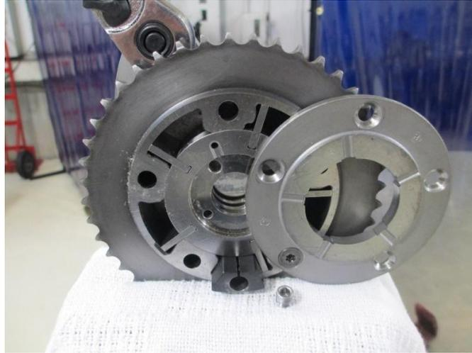
**Step 8:** Place **anti-seize or high-pressure lubricant** on the pipe plug, and thread the plug into the lock. Use your 5/32" Allen socket or wrench to tighten the plug until the lock does not move.
