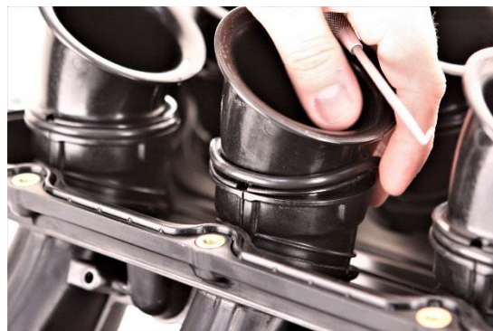
Figure 3 – Photo of the O-Ring above the lip – The stack will be loose now.
