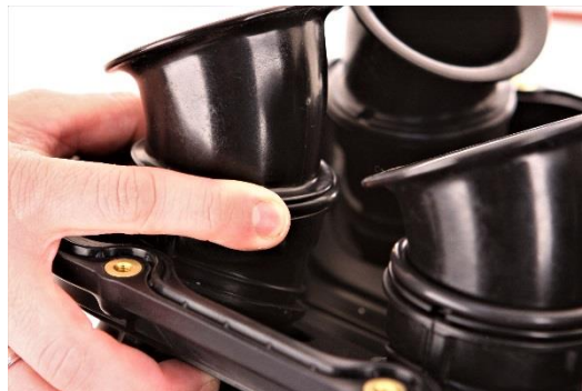
Figure 6- Press the O-Ring evenly in the groove, make sure it's even all the way around.
