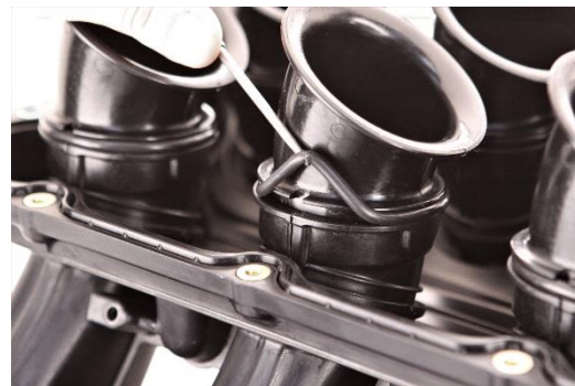
Figure 2 – Pull the O-Ring over the lip on the velocity stack
