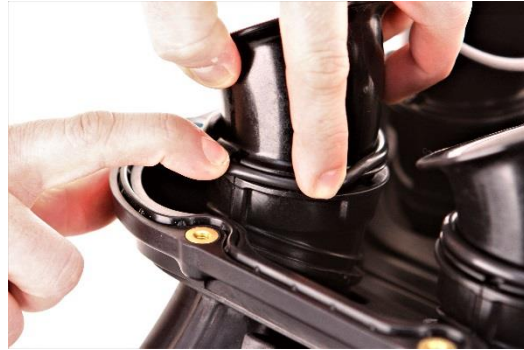
Figure 5 – Holding the runner up in the locking tabs, roll down the O-Ring.
