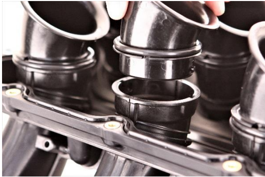
Figure 4 – Align tabs to the slot. See the O-Ring is above the lip.
