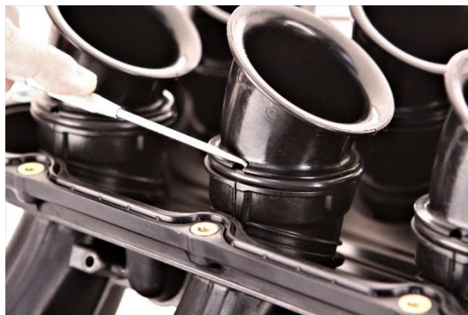
Figure 1 - Insert a 90 degree pick on the back side of the O-ring
