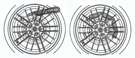
A rotor protector should always be installed before any wheel removal. The protector can be installed by feeding it through the wheel spokes and slipping it over the outer edge of the rotor. Leave the protector in place, over the rotor edge, until the wheel is re-installed. Rotor protectors are available through your dealer/retailer.
