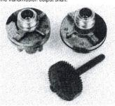
Twelve speedometer driven gears are available for the 4L60 transmission to calibrate the speedometer with various axle ratios and tire diameters.
