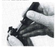
Transfer the wires from the four-pin connector to the respective terminals in the five-pin connector ("A" to "A", "B" to "B", etc.). The fifth "E" terminal is not used.
