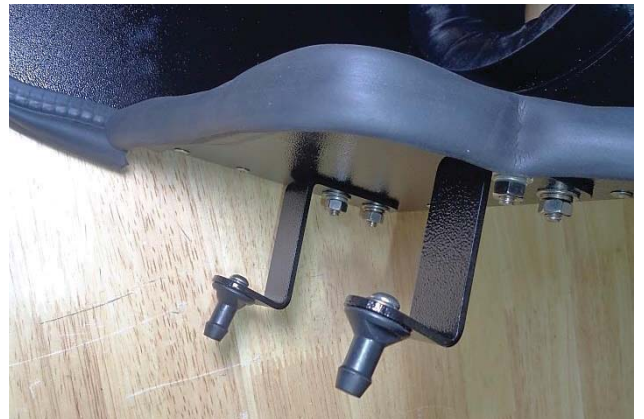
17. Fasten a barbed pin (14) to each bracket, using an M6 screw (13), lock washer (8) and flat washer (7).
