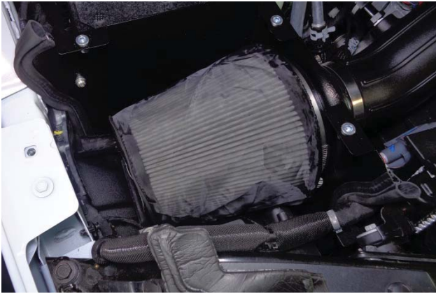
25. Place the pre-filter wrap (28) and the #104 screw clamp (2) on the air filter (1). Then install the filter on the filter adapter, and tighten the clamp.
