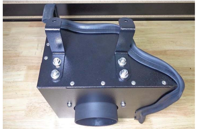
16. Attach the 2 brackets (15) to the heat shield as shown, using ¼-20 screws (10) (against the heat shield), and flat washers (12), lock washers (11), and nuts (16) (against the brackets).
