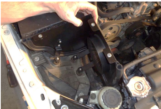
14. Set assembled airbox in vehicle, aligning the 3 barbed pins with their rubber grommets in the vehicle. Adjust alignment of brackets (22) if required. Push each pin into its grommet, one at a time. NOTE: Moistening the grommets with soapy water will ease insertion.
