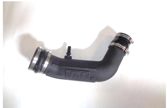
17. Install 2 hose clamps (12) on flex coupler (20), and install coupler on intake end of intake tube. Install hose clamps (15) and (13) on tapered coupler (14), and install coupler on discharge end of tube. Orient clamp screws so as to allow tightening after installation on vehicle.
