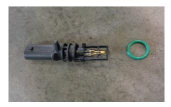
6. Remove the o-ring from the air temperature sensor. Place a sensor-safe grease or lubricant on the o-ring surface to facilitate easier installation into the FM air intake tube grommet. Retain in a safe location.
