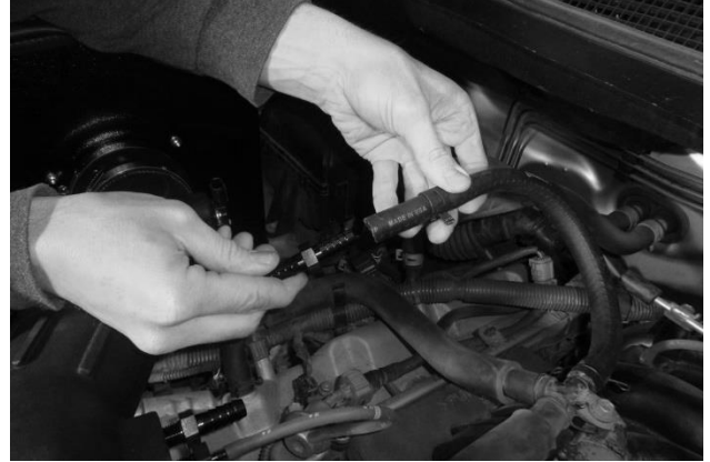
33. Insert barbed fitting (15) into PCV hose and secure with pinch clamp (14).
