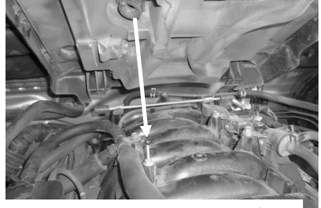
38. Install engine heat shield. Place clips at rear of cover on hinge bar, then lower the cover and snap it into place on the mounting post.
