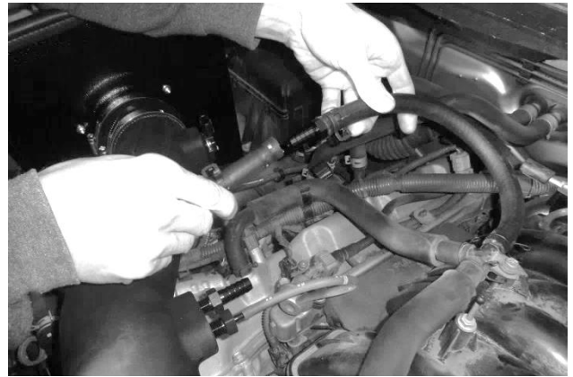
34. Install PCV hose (16) on barbed fitting and secure with pinch clamp (14).
