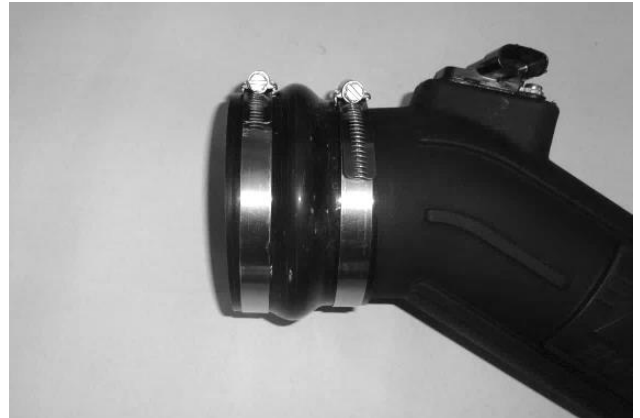
28. Install two hose clamps (22) on flex coupler (11), and install coupler on intake end of intake tube. Orient clamp screws to allow tightening after installation on vehicle.
