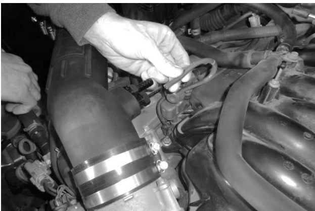
32. Install vacuum hose on small barbed fitting.
