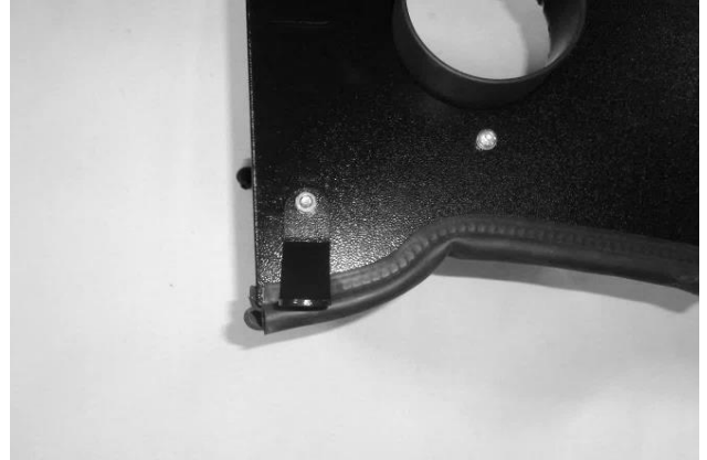
21. Attach bracket (23) to airbox using ¼-20 × 5/8" screw (28) and flat washer (25) (against airbox), and nut (7) and lock washer (8) (against bracket). Leave bracket slightly loose until installation of airbox.
