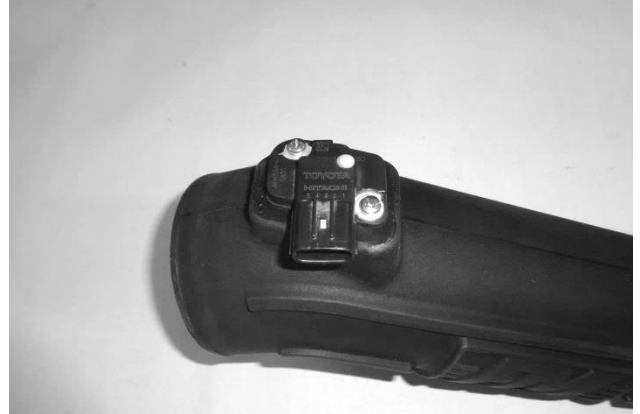
27. Install MAF sensor gasket (12) onto the sensor, ensuring correct orientation. Then install sensor in intake tube, using M4 screws (13).
