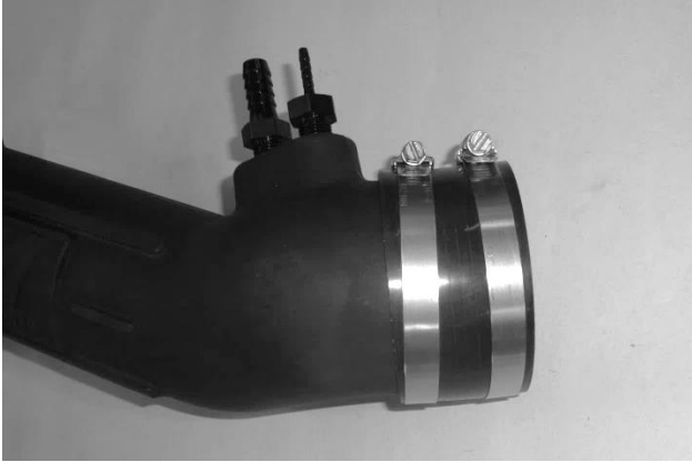
30. Install two hose clamps (21) on straight coupler (20), and install coupler on discharge end of tube. Orient clamp screws so as to allow tightening after installation on vehicle.
