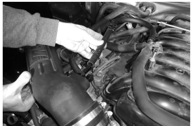
35. Install other end of PCV hose on barbed fitting in intake tube and secure with pinch clamp (14).
