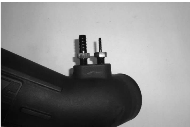
26. Apply 2 wraps of nylon thread tape to threads of barbed fittings (17) and (18), and install them in intake tube (19).
