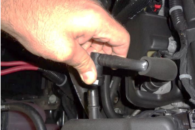
7. Disconnect both PCV hose connectors from the intake plenum by depressing their release latches and pulling straight off.
