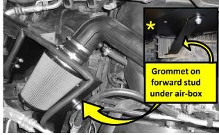
15. Insert the assembled FM intake system into the vehicle as shown\*. Attach the extended crankcase vent hose/clamp. Connect the air temperature sensor plug and secure the intake tube on the throttle body.
