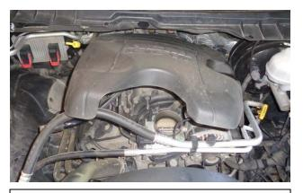
6. Remove the engine cover by grasping the front edge and lifting up and then pulling forward and set aside for reinstallation. It is recommended that you cover the throttle body intake with a clean cloth.
