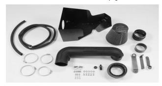
9. Begin assembly of the FM Cold Air Intake System by removing the components and hardware from the packaging and organizing the contents (including the fasteners) by thread and type to avoid confusion.
