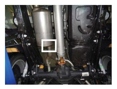
4. Remove bolts attaching muffler and front pipe. Remove grounding wire from muffler.
