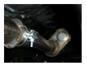
3) Place the provided 3" clamp onto the inlet of muffler **#8530582-258**, then slide onto the factory front pipe and connect the two hangers at the back of the muffler to the rubber mounts on the vehicle. Be sure to line up the notch on the muffler inlet with the tab on the pipe.
