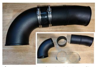
Construct your route from throttle body to air filter location. Each tube connects using a coupler and two clamps as shown. Remember to integrate MAF sensor and Intake Air Temperature (IAT) sensor as well.
