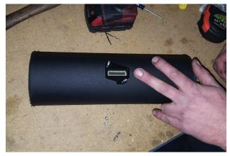
6. Insert screws (x2) (23) (from inside out) through tube and MAF adapter. Outline center slot in adapter onto tube as shown.
