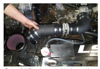
3. Install air filter adapter onto air intake assembly.
