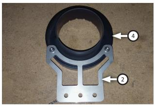
2. Install bracket 1 (2) onto air filter adapter (4) using (x2 ea.) screws (15), flat washers (17) and split lock washers (16).
