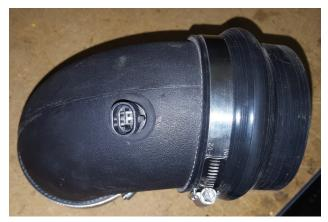
3. Install air intake sensor (removed step 1) in through grommet and tube. Use soapy water to ease insertion if necessary.
