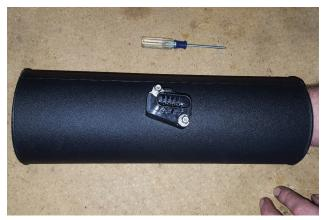
10. Install MAF sensor onto MAF adapter using locknuts (x2) (24).
