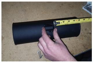
3. Place MAF adapter onto tube and center it. Make sure slot aligns with center line of tube. Adapter should sit perfectly flat.
