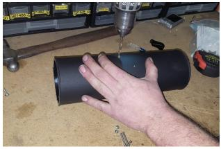
NOTE: Be careful not to oversize or the fastener heads could slip through.
