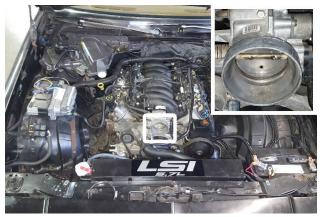
3. Identify throttle body in your vehicle, this will be the starting point for your universal air intake kit. Verify sizing then select appropriate coupler for it (very likely 3¾-4").
