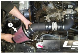
4. Install air filter (3) onto adapter and position it how you would like it to sit.
