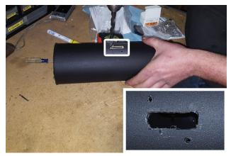
7. Disassemble parts from tube then drill marked slot for MAF Sensor. You can oversize your drill up to an 1/8" so your MAF Sensor slides in and out easily. Deburr and smooth drilled edges.
