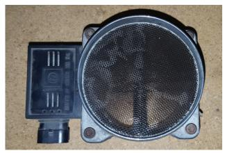
1. This style MAF is housed and will have to be integrated into your tubing assembly. Start by uninstalling housing from vehicle.
