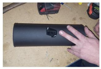
8. Apply RTV to MAF adapter and install it onto tube using (x2 ea) screws to locate it properly. Use locknuts (24) to secure adapter in place then wait for RTV to set (approximately 1 hour).
