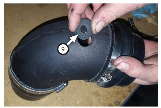
2. Deburr hole then install grommet (9).
