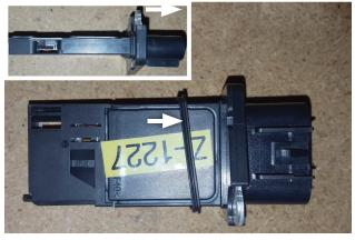
NOTE: Index how factory MAF sensor is oriented in your vehicle. It is important to know so you can properly transfer it into your new intake kit.
