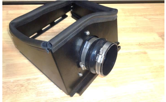
16. Slip the #56 screw clamp (15) onto the small end of a coupler (14), and install the coupler on the filter adapter. Push the coupler up against the heat shield, and tighten the clamp. Then slip the #64 screw clamp (13) onto the other end of the coupler.
