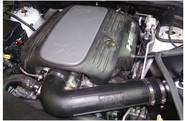
28. Re-install engine cover (removed step 3).
