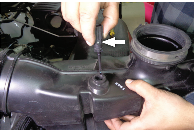
9. Remove IAT sensor from resonator, remove o-ring from IAT sensor then retain sensor for re-use.
