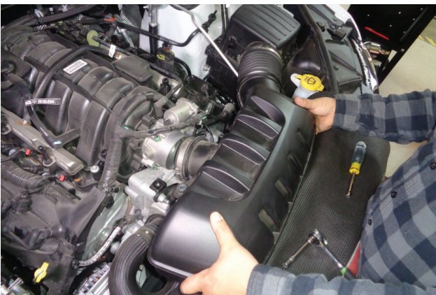
8. Remove resonator from engine compartment.
