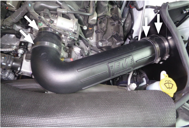
25. Push couplers flush against heat shield and throttle body before fastening outermost screw clamps (x2). Center intake tube between couplers then tighten remaining screw clamps (x2).
