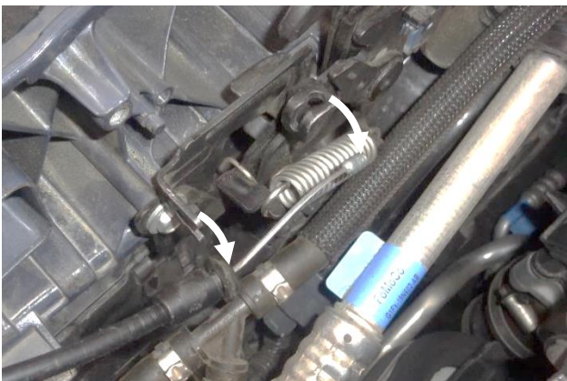
15. Remove the hood release cable end and grommet from the latch mechanism.
