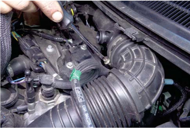
8. Loosen the screw clamp that secures the inlet air duct to the turbo inlet.
