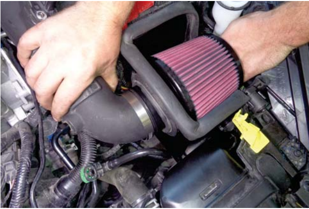
31. Carefully push the air filter (1) through the heat shield gasket and onto the intake tube.
