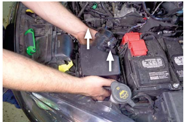
12. Lift the airbox up sharply about 1–2 inches—just enough to release it from its 2 mount grommets.
