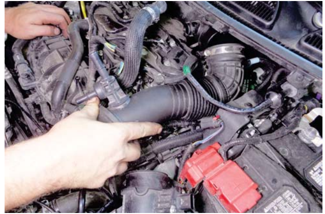
10. Separate the inlet air duct from the airbox and turbo inlet, and remove it from the vehicle.
