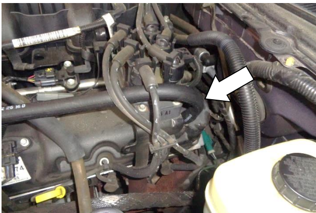
26. Route one end of the 1/2" hose (25) under the spark plug wires and push it onto the PCV port at the rear of the engine.
