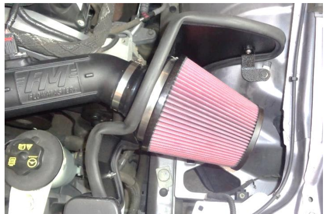
29. Install the clamp (2) on the air filter (1), then install the filter on the filter adapter and tighten the clamp.
