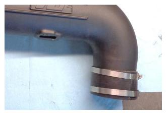
17. Slip the #64 screw clamps (10) onto the coupler (8), and install the coupler on the discharge end of the intake tube. Do not tighten the clamps at this time.
