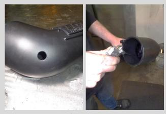
15. Deburr the edge of the hole, and blow any debris out of the intake tube.
