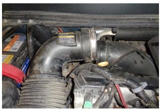
6. Separate the inlet duct from the turbo inlet.
