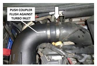
20. Push the coupler flush against the raised lip on the turbo inlet, then tighten the turbo inlet clamp only.
