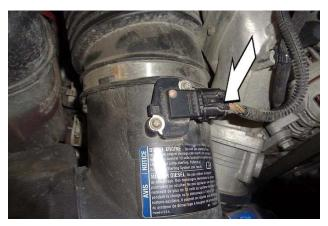
4. Disconnect the plug from the MAF sensor by depressing the locking tab and pulling the plug straight off the sensor.
