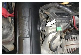
24. Push the MAF sensor plug onto the sensor until the locking tab clicks, then check the plug for security.
