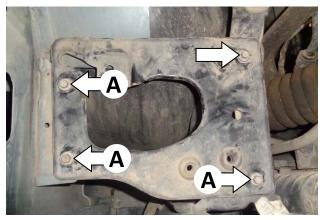
10. Remove the airbox shelf by removing its 4 mount screws. Retain the screws for later use. NOTE: To ensure proper screw clearances at reinstallation, note the length of the screws removed from the 3 locations marked (A) above.
