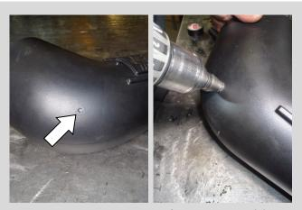
14. At the dimple in the bend of the intake tube (9), drill a 13/16" hole. **NOTE: Use of a step drill is recommended.**
