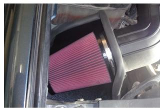
22. Place the #104 screw clamp (2) on the air filter (1), install the filter on the intake tube, and tighten the clamp.
