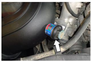
25. If you are using the filter restriction indicator, carefully push it into the grommet. (Moistening the grommet I.D. with soapy water will ease insertion.)
