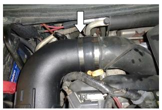
23. Ensure that at least 1/2" of the intake tube extends inside the coupler, then tighten the clamp on the intake tube.
