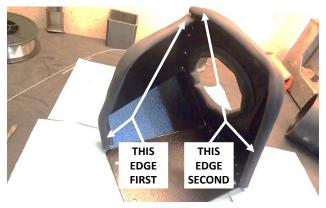
12. Attach the gasket to the two outer edges of the heat shield in the order shown. (Note that the second gasket will overlap the first at the middle corner.) Use metal-cutting shears to trim the gasket to fit.
