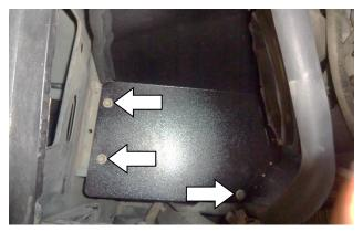
13. Use the 3 screws removed from locations (A) in Step 10 to install the heat shield in the vehicle. NOTE: To maintain proper screw clearances, be sure to use the same length screw at each location as was removed.
