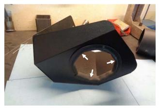
11. Attach the gasket (4) to the I.D. of the heat shield (3) as shown. Firmly press the gasket onto the edge, gradually working all the way around. When you return to the starting point, use metal-cutting shears to trim the gasket to fit.
