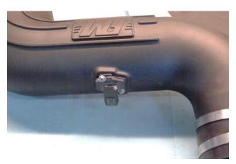
18. Install the MAF sensor gasket (6) over the sensor, then install the sensor in the intake tube, ensuring the correct orientation of the gasket and sensor to the mount pad. Secure the sensor using M4 screws (7).
