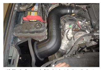
19. Slip the front end of the intake tube into the heat shield, then slip the coupler over the turbo inlet.
