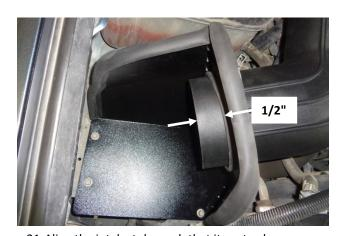
21. Align the intake tube such that it protrudes approximately 1/2" into the heat shield.
