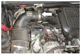
5. Loosen the screw clamp that secures the inlet air duct to the turbocharger inlet.
