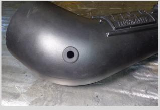
16. Insert the rubber grommet (5) into the hole. (Moistening the hole with soapy water will ease insertion.)
