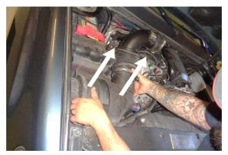
7. Remove the airbox and inlet duct from the vehicle by pulling the airbox firmly straight up to release it from its rubber grommets.
