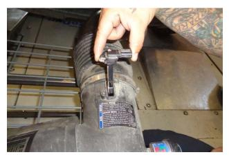
8. Remove the MAF sensor from the airbox, then remove the o-ring from the sensor. CAUTION: The MAF sensor is delicate! Handle it with care, and store it in a safe location until reinstallation.
