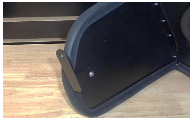
18. Attach bracket (4) to the heat shield using a 1/4-20 screw (8) (on the heat shield side), and a flat washer (5), lock washer (6) and nut (7) (on the bracket side). Do not fully tighten the fasteners at this time.
