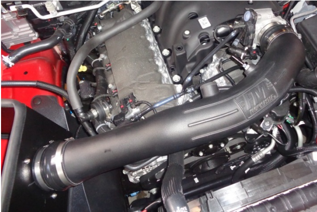
29. Install the intake tube in the vehicle. Do not tighten any screw clamps at this time.
