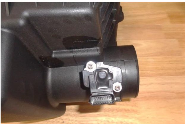
15. Remove the MAF sensor from the airbox, then remove the factory gasket from the sensor. CAUTION: The sensor is delicate! Handle it with care, and store it in a safe location until reinstallation.
