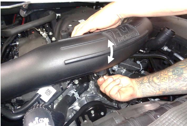
30. Rotate the intake tube as necessary to align it with the bracket. Secure the tube to the bracket with an M6 screw (14), lock washer (13) and flat washer (12).
