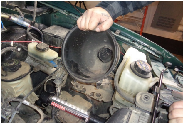
14. Remove the air cleaner from the airbox. Then remove the airbox from the vehicle by firmly pulling it straight up, out of its two mount grommets.
