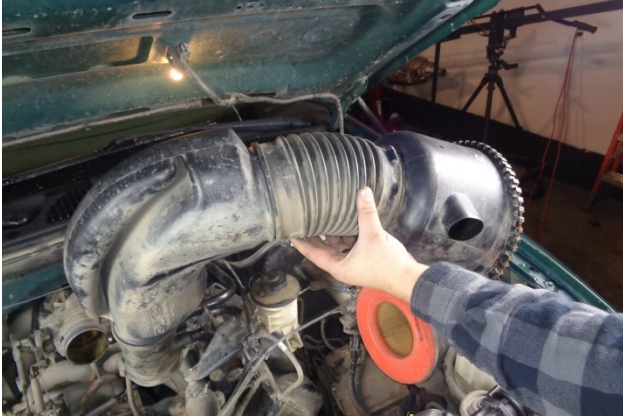
13. After the plug is disconnected from the sensor, remove the inlet duct from the vehicle.
