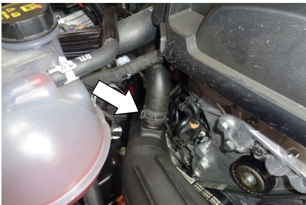
27. Push the diverter valve hose into the intake tube and secure it with the pinch clamp.
