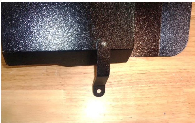
15. Attach bracket (16) to the heat shield using a 1/4-20 screw (8) (against the bracket), and a flat washer (10), lock washer (11) and nut (12) (against the heat shield). Do not tighten the bracket fasteners at this time.
