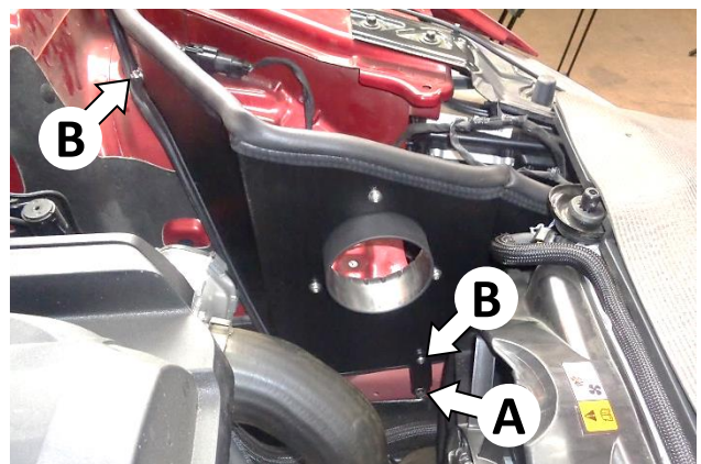
18. At the lower front bracket (A), install and tighten the M8 bolt (15), lock washer (14) and flat washer (13). Then tighten the fasteners (B) holding each bracket to the heat shield.
