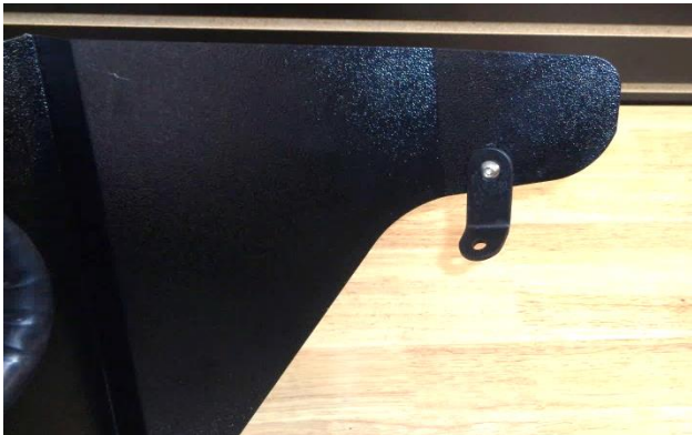
14. Attach bracket (9) to the heat shield using a 1/4-20 screw (8) (against the bracket), and a flat washer (10), lock washer (11) and nut (12) (against the heat shield). Do not tighten the bracket fasteners at this time.
