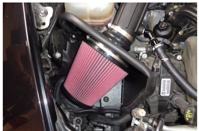
29. Slip screw clamp (2) onto air filter (1), then install the filter on the filter adapter and tighten the clamp.
