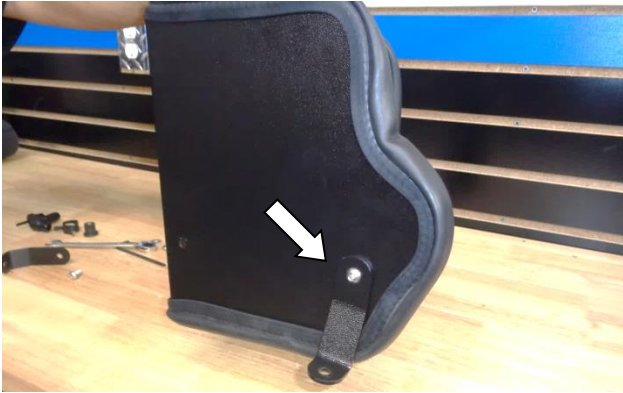
13. Attach bracket (6) to the heat shield using a ¼-20 screw (9) (on the bracket side), and flat washer (10), lock washer (11) and nut (12) (on the heat shield side). Do not fully tighten the fasteners at this time.
