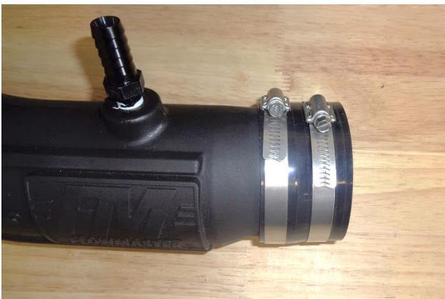
21. Install the two small screw clamps (23) on the small coupler (24), and install the coupler on the throttle body end of the intake tube. Do not tighten clamps at this time.
