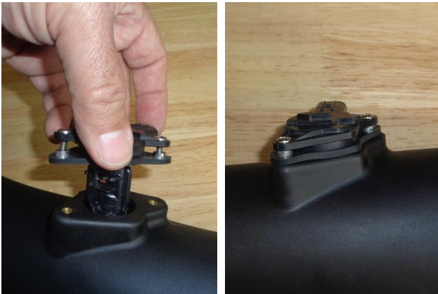
20. Install the assembled sensor, gasket and spacers in the intake tube using M4 screws (25).
