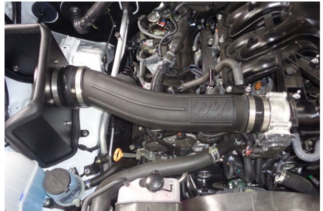
23. Install the intake tube between the heat shield and the throttle body.
