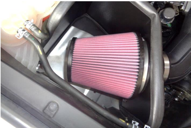
26. Place the clamp (2) on the air filter (1), install the filter on the filter adapter and tighten the clamp.
