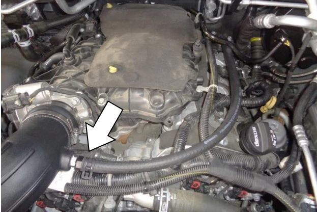
25. Route the hose to the 1/2" barbed fitting, cut it to the desired length, and secure it to the fitting with the pinch clamp (24).
