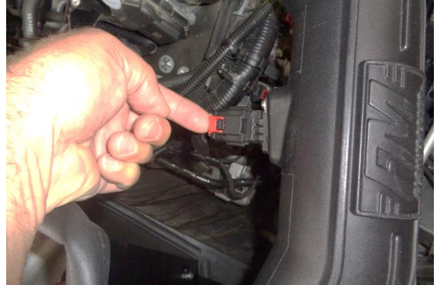
27. Reconnect the MAF sensor plug to the sensor, push the locking tab toward the sensor, and check the plug for security.
