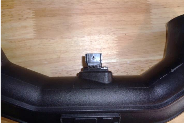
19. Install the MAF sensor gasket (19) on the sensor, ensuring correct orientation. Then install the sensor in the intake tube (22), using M4 screws (18). Tighten the screws evenly for a good seal.
