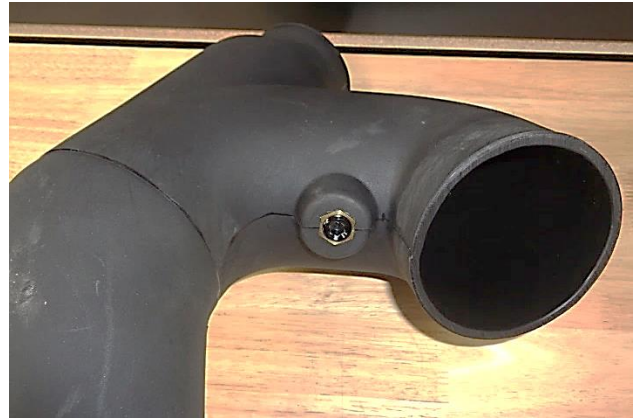
15. Apply 2 wraps of nylon thread tape to the threads of the plug (13), and install it in the intake tube.
