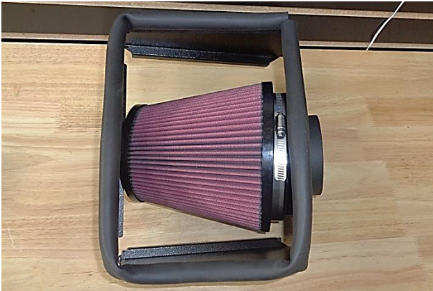
12. Slip screw clamp (2) onto air filter (1), then install the filter on the filter adapter and tighten the clamp.
