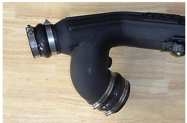
16. Slip the two small screw clamps (16) onto the 3" flex coupler (15). Slip two large screw clamps (10) onto a 4" flex coupler (11). Push each coupler onto the intake tube, and snug – do not tighten – only the tube clamps at this time. (Leave the other clamps loose.)
