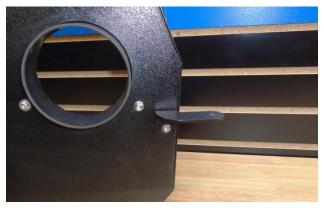
13.Attach bracket (18) to the heat shield using a  $\frac{1}{4}$ -20  $\times$  5/8" screw (23) (against the bracket), and a flat washer (19), lock washer (20) and nut (21) (against the heat shield). **Do not tighten the bracket fasteners at this time.**
