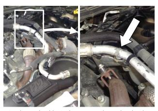
24. The stock cable tie that secures the coolant hard line may break during removal of the stock intake system. Your kit includes a fourth cable tie (24) to replace the stock part, if needed.
