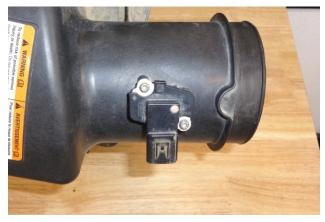
Remove the MAF sensor from the airbox, then remove the factory gasket from the sensor.
