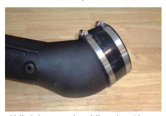
20. Slip the larger screw clamps (13) onto the straight coupler (12). Install the coupler on the oval end of the intake tube. Only snug – do not tighten – the tube clamp at this time. (Leave the other clamp loose.)
