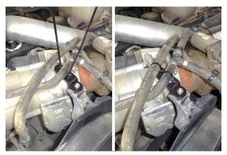
23. Attach bracket (22) to the mount point for the stock intake duct, using an M6 screw (8), lock washer (7) and flat washer (6). Then secure the two hoses to the bracket using two cable ties (24).
