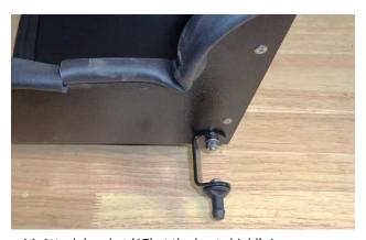
14. Attach bracket (17) at the heat shield's inner corner using a %-20  $\times$  5/8" screw (23) and flat washer (19) (against the heat shield), and a lock washer (20) and nut (21) (against the bracket). Then attach a barbed pin (14) to the bracket, using an M6 screw (8), lock washer (7) and flat washer (6).
