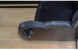
15. Attach a barbed pin (14) to the heat shield's outer corner using and M6 screw (8), lock washer (7) and flat washer (6).
