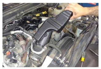
10. Separate the intake duct from the turbo inlet, then remove the duct from the vehicle.
