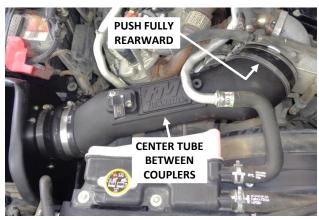
21. Install the assembled intake tube in the vehicle.
