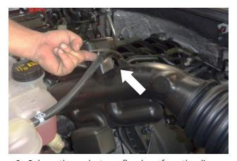
6. Release the coolant overflow hose from the clip on top of the intake duct.
