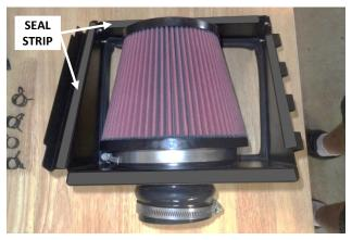
13. Slip clamp (2) onto air filter (1), install filter on filter adapter, and tighten clamp. Cut adhesive seal strip (4) to the lengths required, and apply to the four edges of the heat shield.
