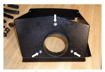
10. Assemble air filter adapter (3) to heat shield (17) using M6 screws (15), lock washers (6) and flat washers (5).
