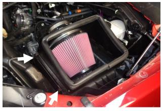
14. Place the assembled heat shield on the airbox, and secure it with the two locking clips.
