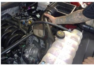
9. Carefully remove the intake duct from the vehicle.
