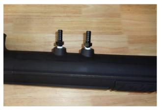
15. Apply 2 wraps of nylon thread tape to the threads of the two 1/2" barbed fittings (9), and install them in the intake tube (8).
