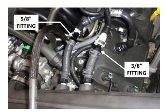
20. Cut the 1/2" hose (11) approximately in half, and clamp the 5/8" fitting (12) in one of the two hoses with a pinch clamp (14). Insert the fitting into the PCV connector, cut the hose to reach its barbed fitting on the intake duct, and secure the hose to the fitting with a pinch clamp (14). Repeat the process for the 3/8" fitting (13) and the EVAP connector.
