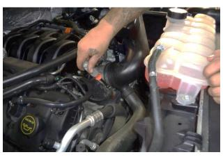
8. Loosen the hose clamp securing the air intake duct to the throttle body, then disconnect the intake duct from the throttle body.
