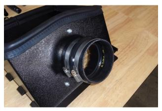
12. Slip two hose clamps (7) onto a coupler (10). Push the coupler onto the air filter adapter, all the way against the heat shield, and tighten the clamp.
