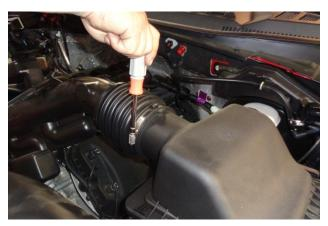
4. Loosen the hose clamp securing the air intake duct to the airbox cover, then disconnect the intake duct from the airbox cover.
