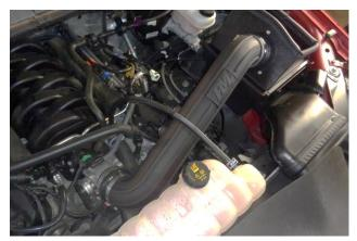
19. Install the intake tube in the vehicle. (The tube will pass under the coolant overflow line.) Push the coupling up against the throttle body opening and tighten the throttle body clamp. Then check that the tube is properly aligned in both couplings, and tighten the last two clamps.
