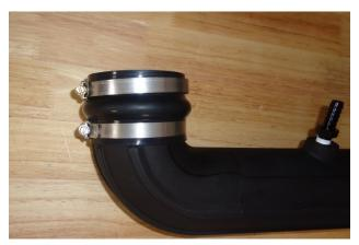
16. Slip two hose clamps (7) onto the other coupler (10). Push the coupler onto the air intake tube and snug (but do not yet tighten) the clamp.
