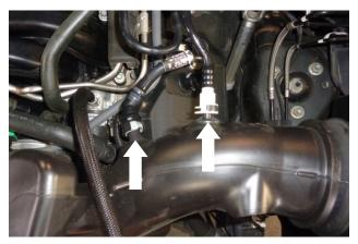
7. Disconnect the PCV and EVAP lines from the intake duct.
