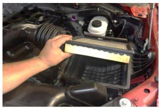
5. Release the two airbox cover clips, then remove the airbox cover and stock air filter.
