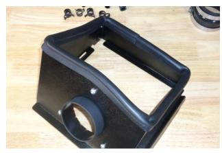
11. Attach gasket (16) to heat shield. Starting in the middle of the edge opposite the filter adapter, firmly press the gasket onto the heat shield, gradually working your way around. When you return to the start point, use metal-cutting shears to trim the gasket to length.
