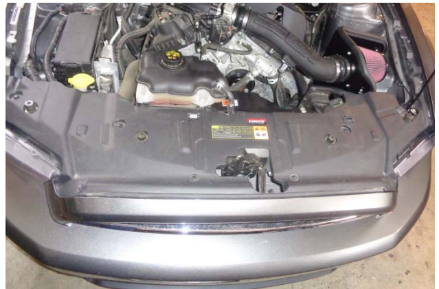
35. Reinstall the radiator support cover and secure with the 6 fasteners (removed at Step 13).
