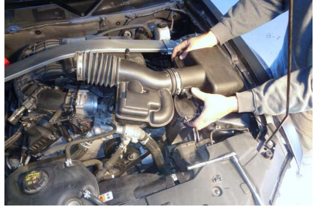
10. Remove the assembled airbox and duct from the vehicle.
