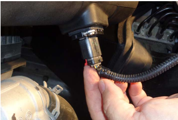
32. Plug the MAF sensor lead into the sensor, push the latch in, and verify the connector is secure.
