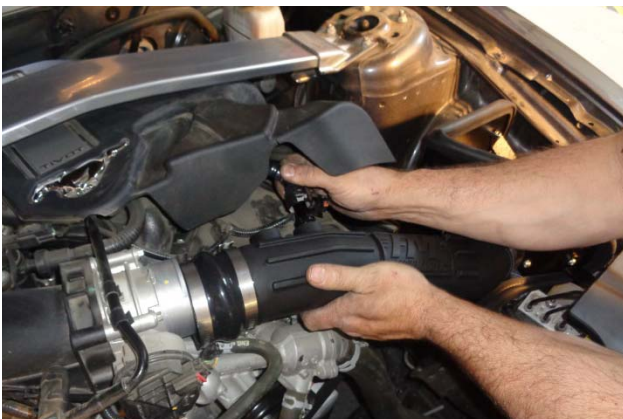
27. Then connect the vacuum hose(s) to their respective fitting(s).
