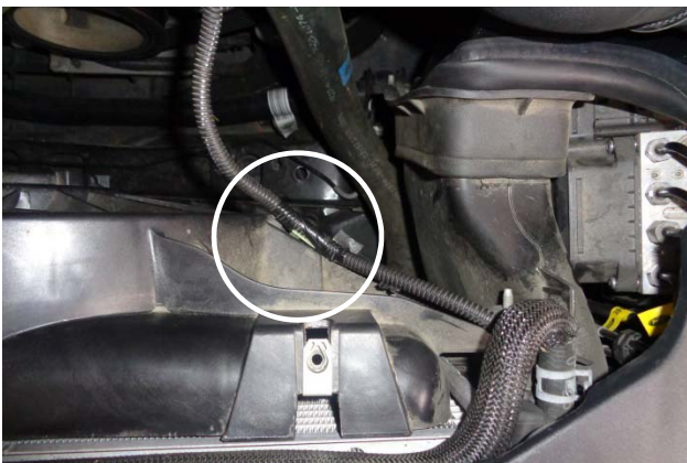
33. Secure the loose MAF sensor lead away from any moving parts, using the factory clip or cable ties.
