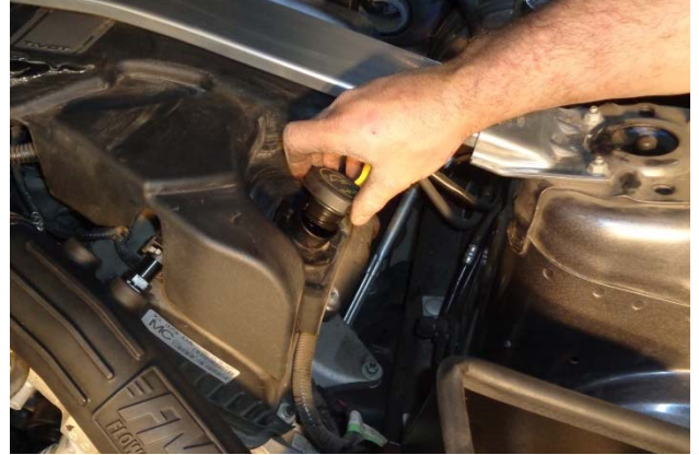
34. If your vehicle includes the optional engine cover, remove the oil fill cap, reinstall the fill cap extension (removed at Step 4), then reinstall the fill cap.
