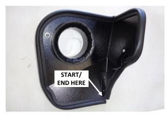
13. Attach gasket (23) to heat shield. Starting at the corner shown, firmly press the gasket onto the edge, gradually working around the heat shield. When you return to the starting point, trim the gasket to fit using metal-cutting shears.
