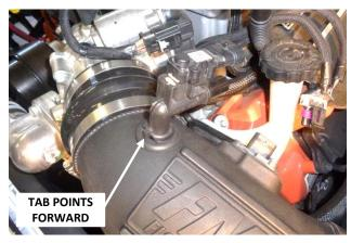
19. Carefully insert the pressure sensor-PCV fitting into the grommet, ensuring that the tab points toward the front of the vehicle. (NOTE: Moistening the grommet hole with soapy water will ease insertion.)
