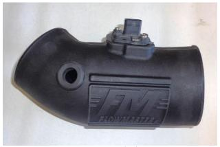
16. Slip the MAF sensor gasket (18) over the sensor, ensuring correct orientation. Then install the sensor in intake tube (14), using M4 screws (19). Install rubber grommet (17) in intake tube.
