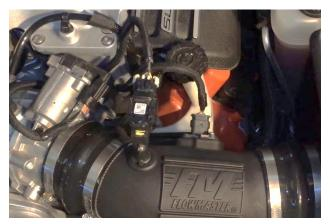
21. Plug the pressure sensor connector into the sensor until it clicks. Plug the MAF sensor connector into the sensor, then press its latch toward the sensor. Verify both connections are secure.
