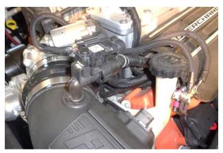
20. Reconnect the PCV hose to the PCV fitting, and verify the connection is secure.
