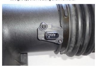
Remove the MAF sensor from the intake duct, then remove the stock gasket from the sensor.
