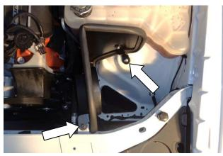
15. Place assembled heat shield in the vehicle. If required, adjust alignment of brackets and retighten their fasteners. Tighten screw (22) at rear bracket, and secure front bracket with **stock bolt removed at Step 6.**
