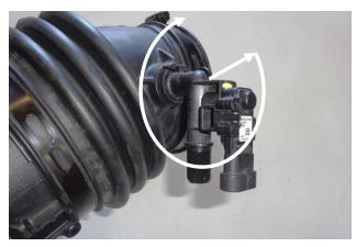
9. To remove the pressure sensor-PCV fitting, firmly grasp it and carefully wiggle it around while pulling away from the duct. (NOTE: Spraying the fitting with penetrating oil from inside the duct will aid removal.) CAUTION: The sensor is delicate! Handle with care, and store in a safe location until reinstallation.
