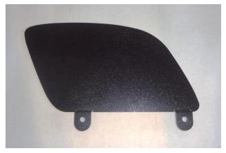
If the vehicle is to be driven in wet weather, it is recommended that the hood intake block-off plate (24) be installed over the intake grille to protect the air filter from exposure to excess water.
