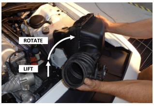
7. Carefully remove the assembled airbox and intake duct from the vehicle by disconnecting the duct from the throttle body, lifting the airbox and duct straight up, then rotating them forward.
