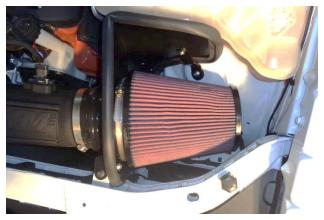
22. Place clamp (2) on air filter (1), install filter on filter adapter and tighten clamp.
