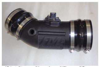
17. Install two small hose clamps (15) on small flex coupler (16), and install coupler on discharge end of intake tube. Install two large hose clamps (13) on large flex coupler (20), and install coupler on intake end of tube.
