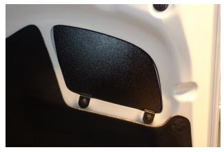
24. Install the block-off plate using the two bolts.
