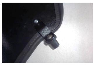
14. Attach rubber rivet nut (5) to bracket (4) with %-16 screw (22), hand tight only.
