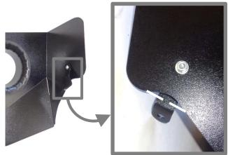
12. Attach bracket (4) to heat shield using ¼-20 screw (6) (against the bracket), and flat washer (7), lock washer (9) and nut (10) (against the heat shield).
