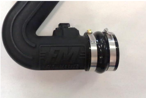
19. Install 2 larger hose clamps (14) on flexible coupler (22), then install coupler on filter end of intake tube.
