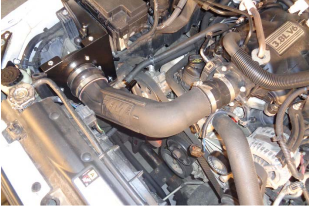
19. Remove the rag or plastic bag (temporarily installed at Step 8) from the throttle body opening. Install assembled intake tube in vehicle and tighten all hose clamps.
