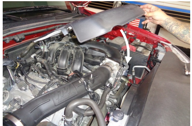
41. Reinstall the engine appearance cover and secure it with the stock nuts.
