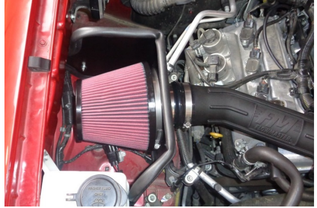
40. Place clamp (2) on air filter (1), install the filter on the filter adapter, and tighten the clamp.
