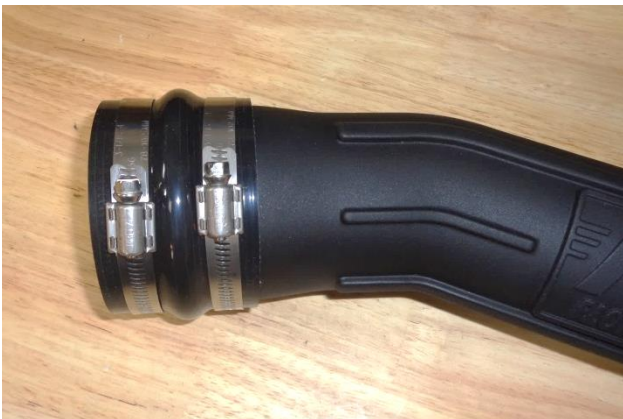
26. Install the 2 large hose clamps (24) on the flex coupler (23), and install the coupler on the filter end of the intake tube. Do not tighten clamps at this time.
