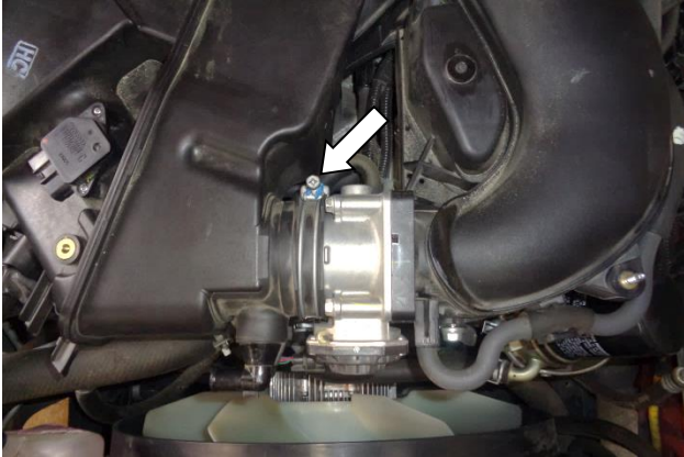
13. Loosen the hose clamp securing the airbox to the throttle body.
