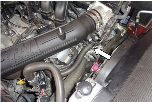
38. Push the PCV hose onto the barbed elbow and secure with pinch clamp (26).
