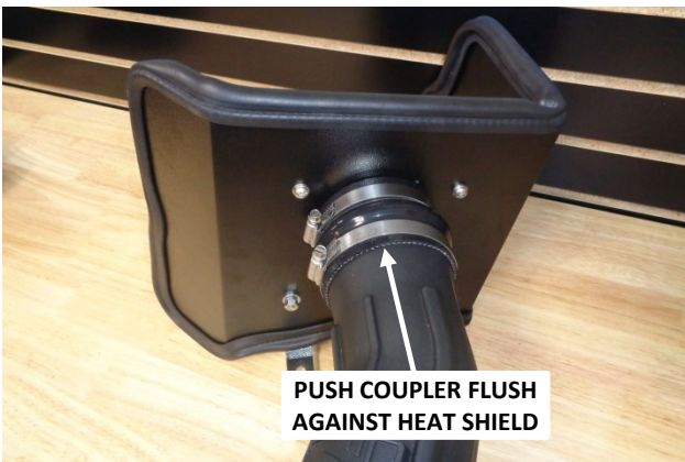
27. Assemble the heat shield and intake tube, pushing the coupler flush against the heat shield. Tighten the clamp at the filter adapter, but only snug the other clamp at this time.
