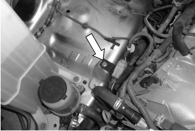
13. Remove nut from harness bracket on wheel well and retain for reinstallation.
