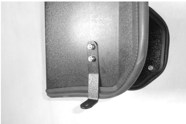
19. Attach bracket (5) to airbox using \frac{1}{4} -20 \times 5/8" screws (3) and flat washers (4) (against airbox), and nuts (7) and lock washers (6) (against bracket).
