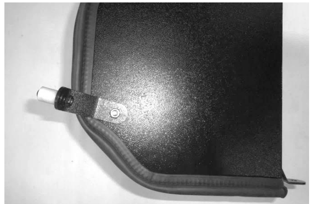
22. Attach bracket (27) to airbox using \frac{1}{4} -20 \times 5/8" screw (3) and flat washer (4) (against airbox), and nut (7) and lock washer (6) (against bracket). Leave bracket slightly loose until installation of airbox.
