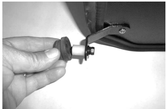
23. Attach nylon spacer (28) to bracket using \frac{1}{4} -20 \times 1 \frac{1}{2} " screw (26), lock washer (6) and flat washer (4) (against bracket), and nut (7) (against spacer). Install rubber bushing on spacer.
