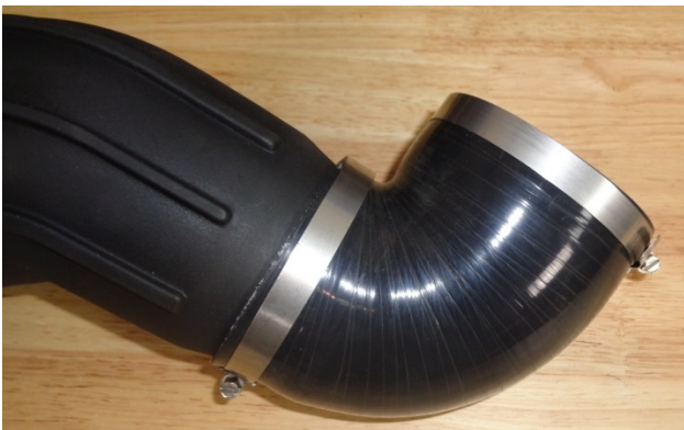
21. Install the small screw clamp (17) on the elbow coupler (18), install the coupler on the other end of the tube, and snug (but do not yet tighten) the clamp. Then slip the last large screw clamp on the other end of the coupler, but do not tighten it yet.
