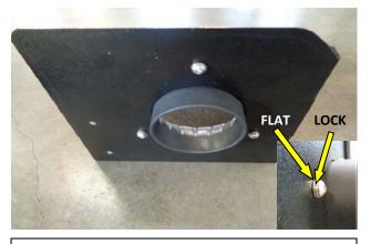
8. Begin by installing the air-filter adapter onto the heat shield as shown. Fasten with three 6mm screws placing the flat and locking washers in the sequence shown. Tighten securely but avoid over-torque.
