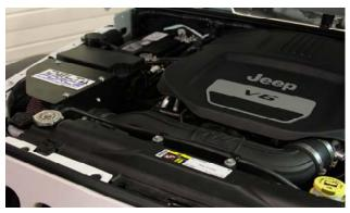
17. Secure the provided cone filter using the included hose clamp in the desired position. Using the last three ¼" screws/washers, secure the air-box lid, reinstall the engine cover and the battery cable. Enjoy!
