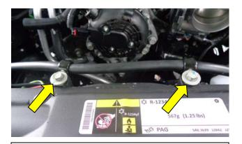
14. Use the retained stock front cross-frame air tube/resonator bolts and the provided vinyl coated loom-clamps to secure the coolant overflow tube to the cross-frame. Do not over-tighten.
