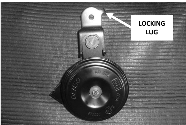
15. On the horn bracket, bend the locking lug flat.
