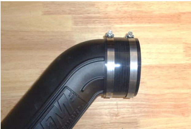
20. Install the two large screw clamps (16) on the straight coupler (17), and install the coupler on the large end of the intake tube. Do not tighten the clamps at this time.
