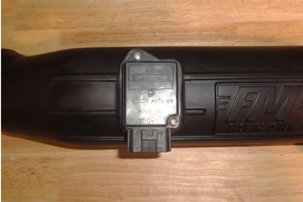
19. Remove the o-ring from the MAF sensor, then install the sensor and gasket (20) on the intake tube using the M4 screws (21).
