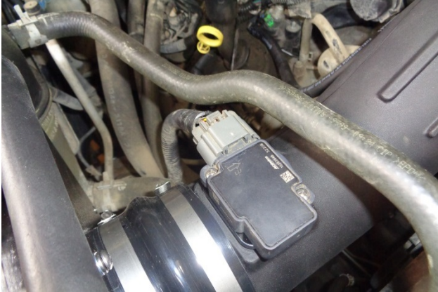
25. Push the MAF sensor plug onto the sensor until it clicks, then verify the connection is secure.
