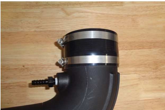
20. Install the other two screw clamps (8) on the straight coupler (9), and install the coupler on the throttle body end of the tube. Snug (but do not yet tighten) just the clamp on the tube.
