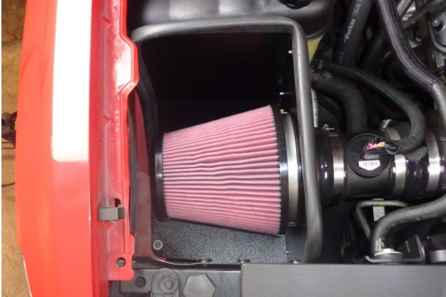
30. Slip clamp (2) onto air filter (1), install filter on filter adapter, and tighten clamp.
