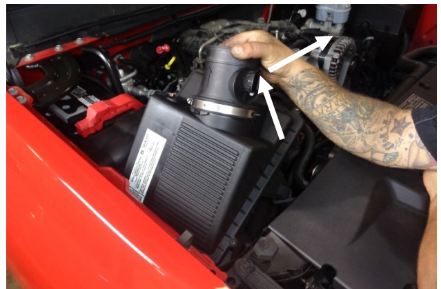
12. Remove the assembled airbox and MAF sensor by grasping the sensor and lifting straight up (to release the airbox mount pins from their rubber grommets), then sliding the airbox inboard to release it from its shelf.
