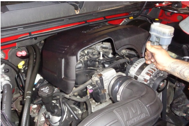
31. Install the engine cover by aligning it with its mount posts, then snapping it into place.
