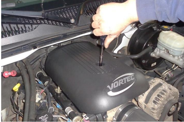
22. Reinstall the engine heat shield.
